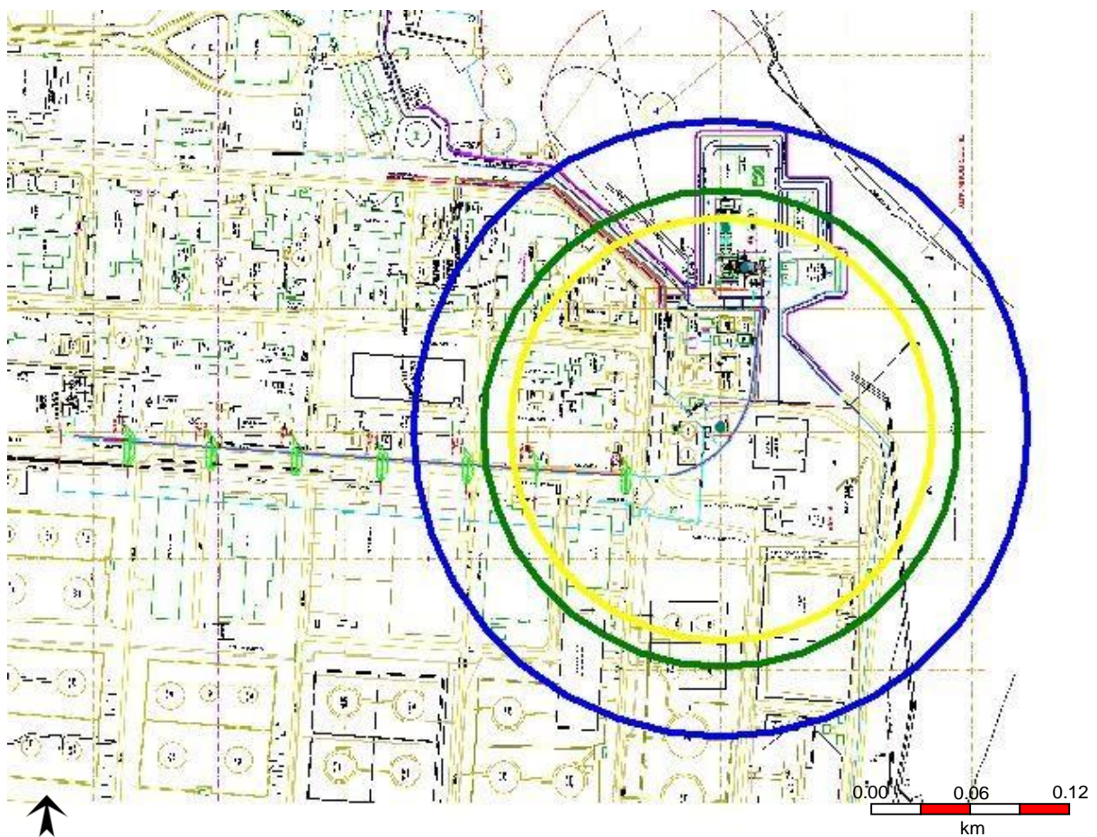
Fig. 8.7 Over pressure damage distance for 100 mm leak of LDO Storage tank
