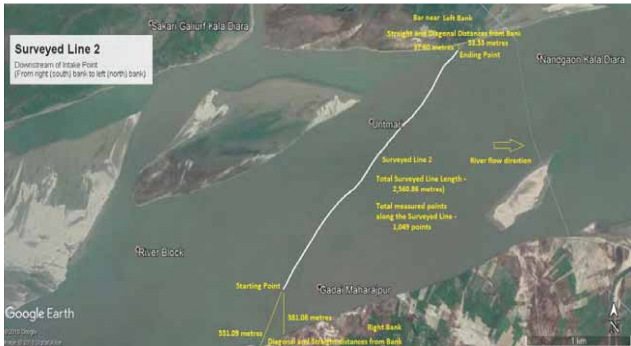
FIGURE 6.58: BATHYMETRIC SURVEY AT CROSS SECTION 2 OF RIVER GANGA – DOWNSTREAM SITE
