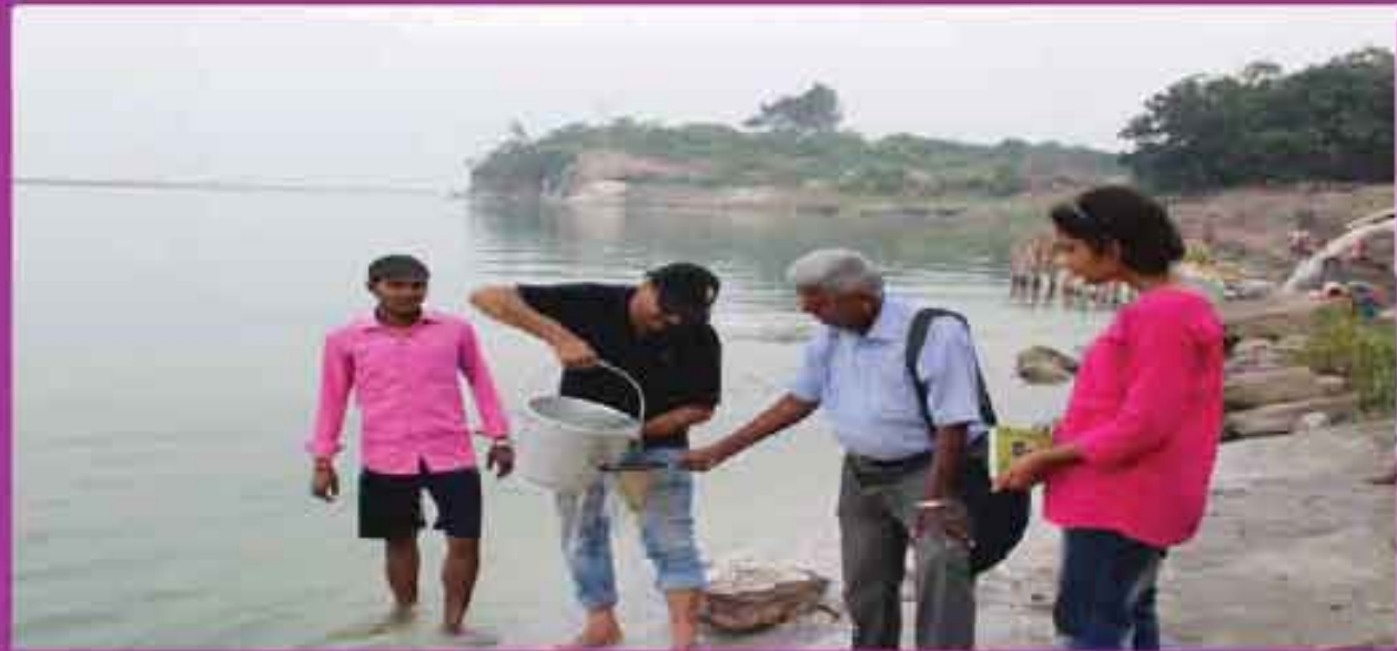
P20: Plankton Sampling at D/S of Proposed Water Intake Site of GTPP
