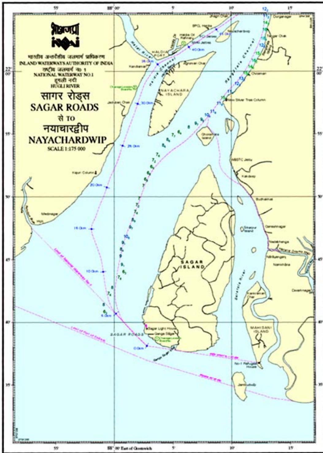
Fig. 3A. Sagar to Nayachar stretch of National Waterway No. 1 (The notations along the water way namely 6 3 , 8 4 , etc. represent water depth as 6.3 m, 8.4 m and so on)
