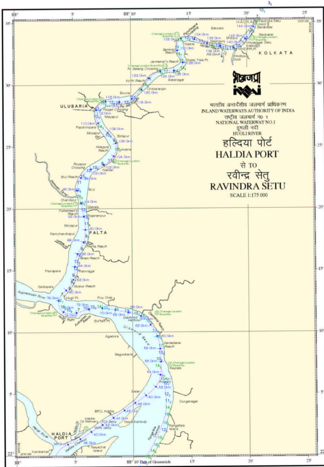
Fig. 3B. Nayachar to Ravindra Setu (Kolkata) stretch of National Waterway No. 1 (The notations along the water way namely 6 3 , 8 4 , etc. represent water depth as 6.3 m, 8.4 m and so on)
