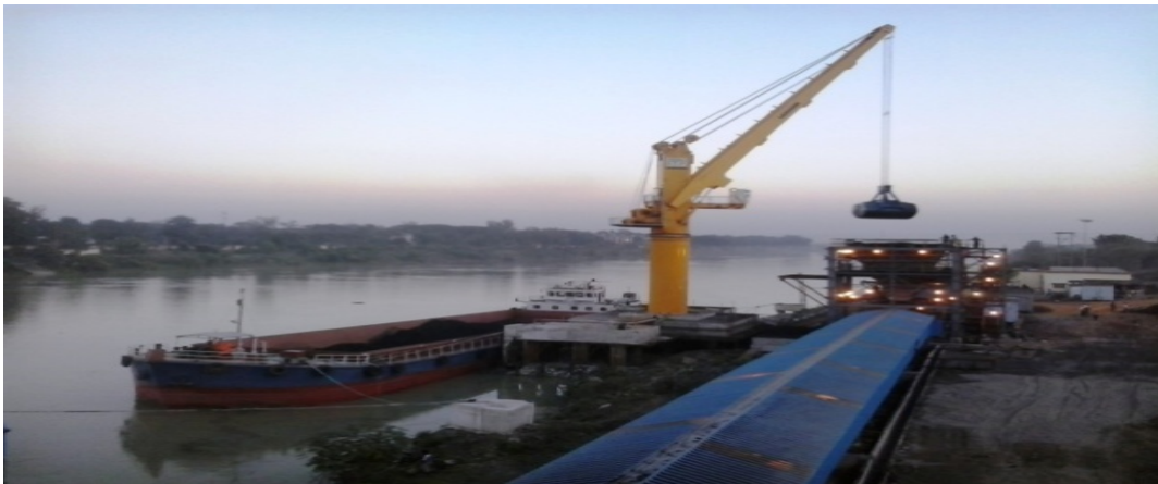
Fig. 9. Coal being unloaded from barge and loaded on to the conveyer system
