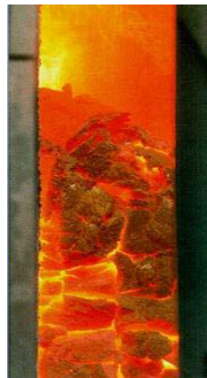
Figure 3-4: Incandescent coke in the oven waiting to be "pushed"
