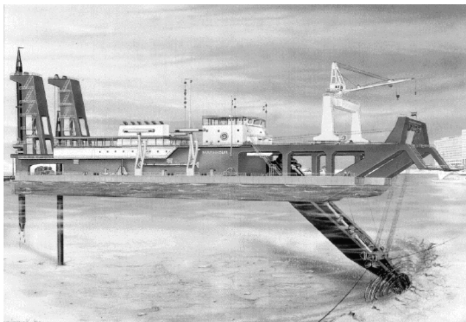
Figure 7-2: Typical cutter suction Dredger
