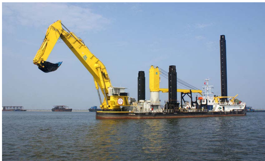
Figure 7-3: Typical backhoe dredger
