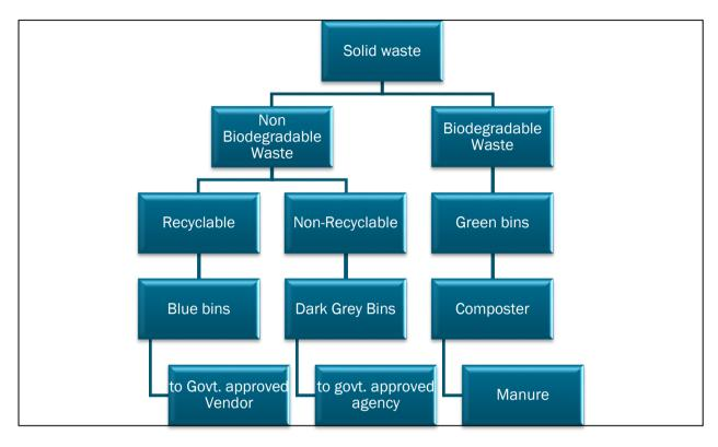
Figure 8: Solid Waste Management Scheme -Domestic Waste
