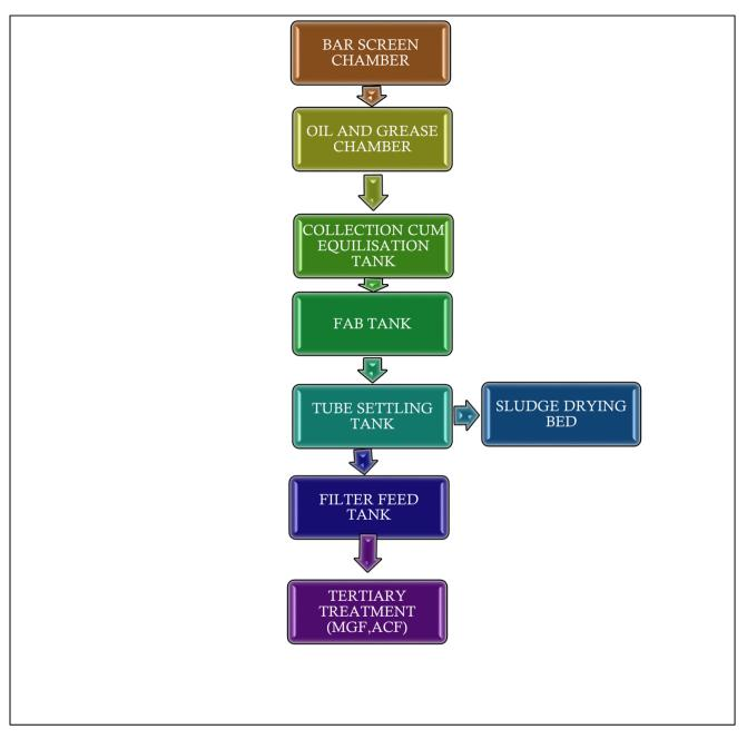
Figure 4-Process and Instrumentation of STP technology
