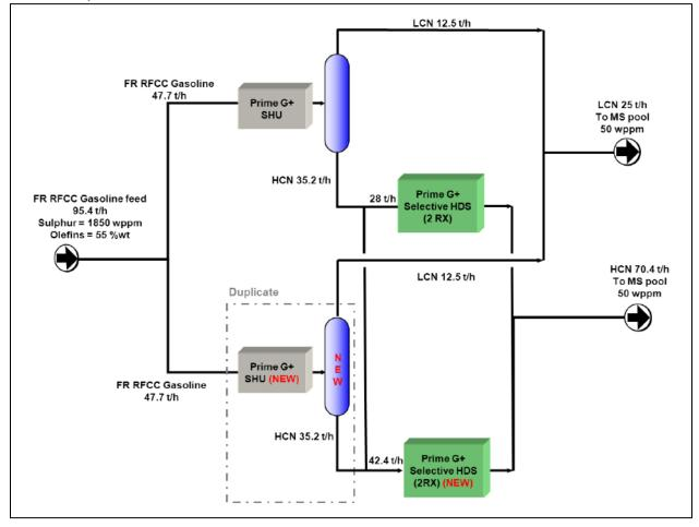
Owing to the important increase in capacity (+ 90%), a new SHU and Splitter section and a new first-stage HDS section operating in parallel with the exiting sections are specified.
