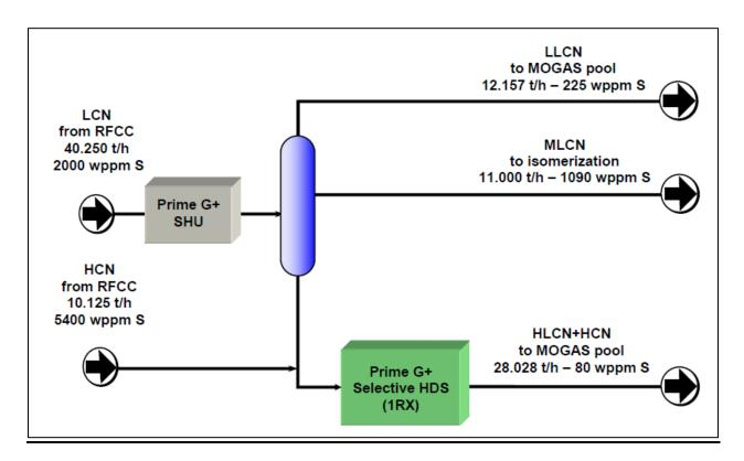
At PDP stage, 10% overdesign was considered on unit feed capacity. Current design capacity of SHU section is thus 44.275 tons/hr and current design capacity of HDS section is 30.938 t/h.
