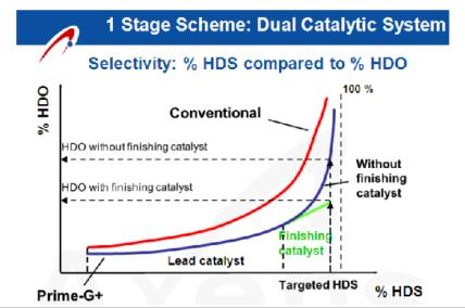
As compared to a conventional hydrodesulphurization catalyst, the lead HDS catalyst (main reactor) ensures a reduced HDO rate for the same HDS rate. The finishing catalyst enables completing HDS with almost no HDO. In addition, finishing reactor features excellent mercaptans control by getting rid of
