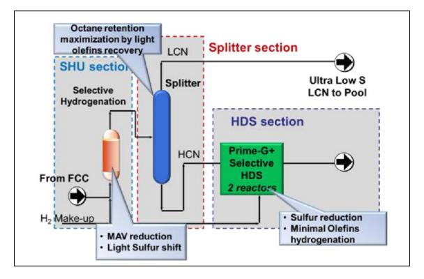
The heavy cut (HCN) is deeply desulphurized with minimum olefins saturation in in Prime-G+TM selective HDS section. Selective HDS section with two reactors relies on Axens dual catalytic system, whose principle is summarized in the figure below.
