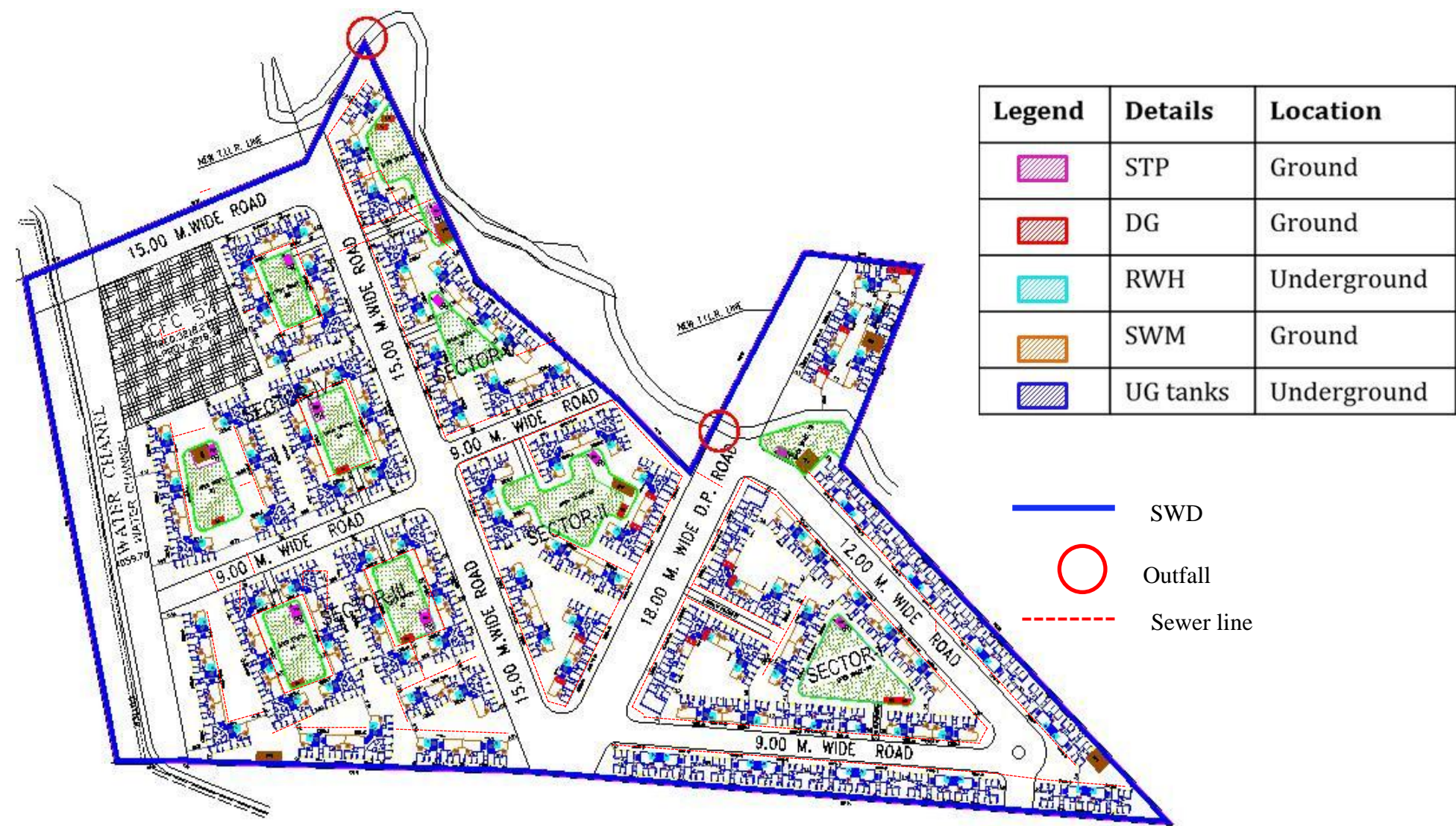
Figure 3: Coordinated layout with landscape, location of STP, SWM, RWH, SWD UG tanks and sewer line
