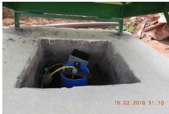
Photo showing piezometer no 8/8 installed near etp-4 of Sukinda mines (Chromite)
