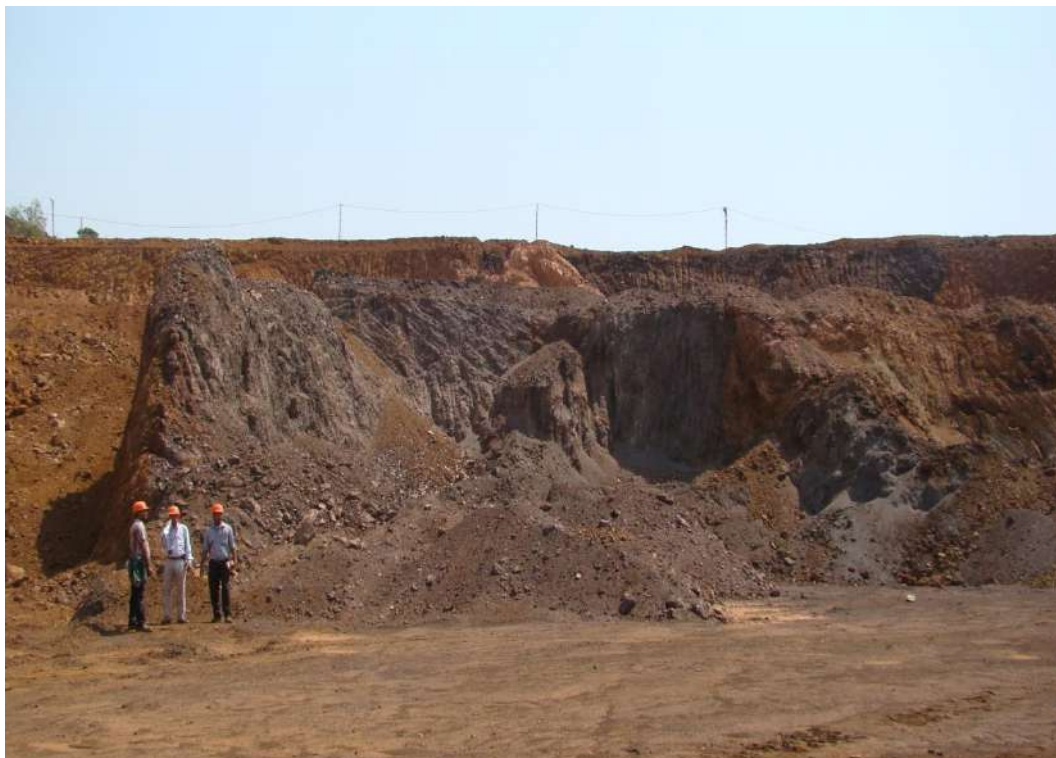
Figure 4.4. Friable chromite ore in the open pit area
