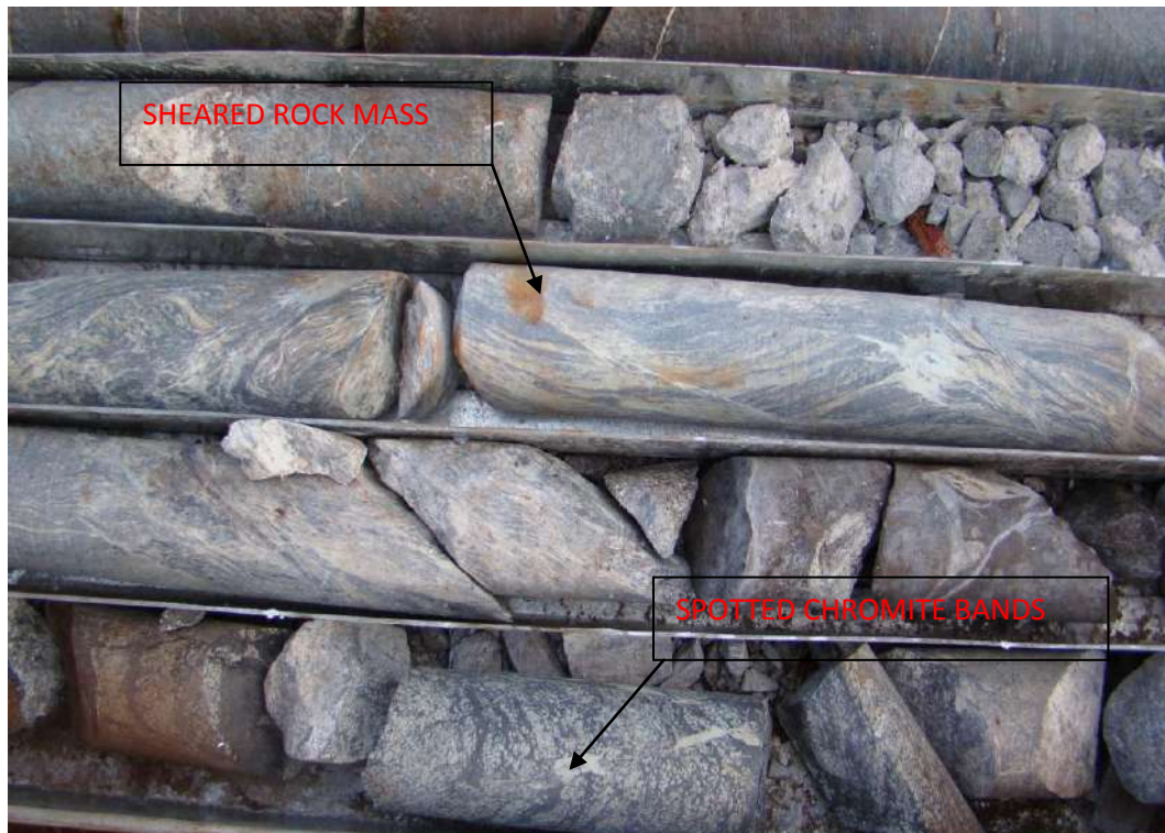
Figure 4.3. Sheared serpentinite and spotted chromite band
