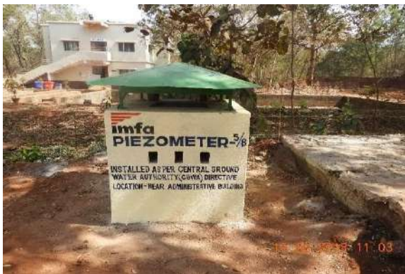
Photo showing piezometer no. 5/8 installed near administrative building of Sukinda mines (chromite)
