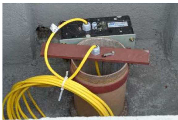
Photo showing Piezometer no. 2/8 installed at near weighbridge of Sukinda mines (Chromite)
