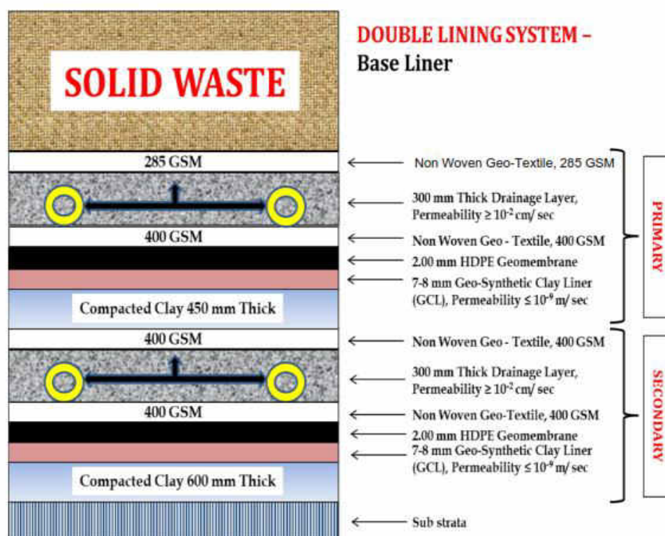
Figure No. 2.11: Double Lining System (Base Liner)
