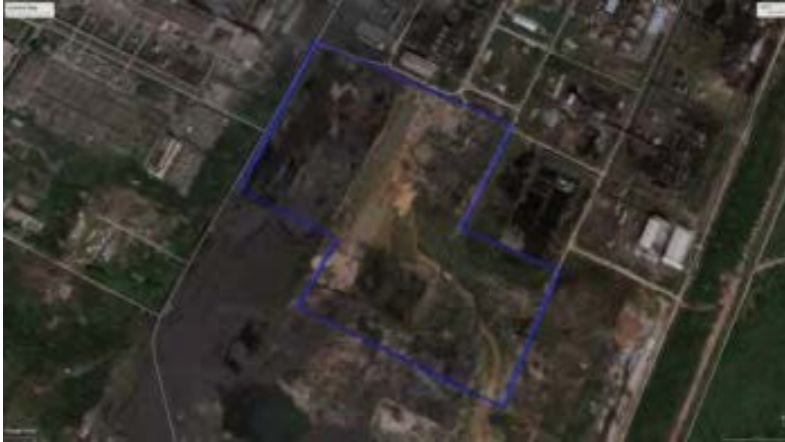
Figure 1.20 : Google Earth Image of 10th Jan., 2016 of Site of COB-5 inside Visakhapatnam Steel Plant (Coal Stock in SW part of Site Completely Cleared. Coal stock in NW part of Mostly Cleared. Civil Works at Site in Progress)
