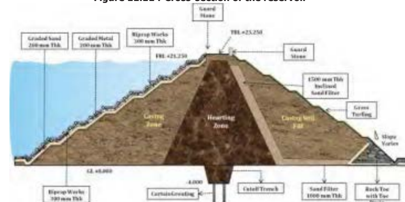
Figure 11.11 : Cross-section of the reservoir
