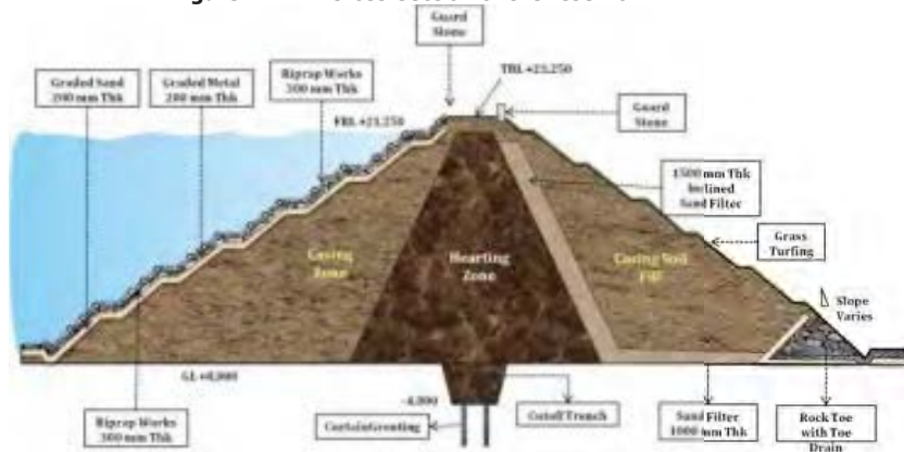
Figure 1.12 : Cross-section of the reservoir
