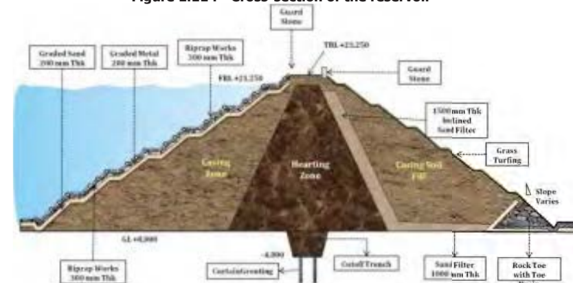
Figure 1.11 : Cross-section of the reservoir
