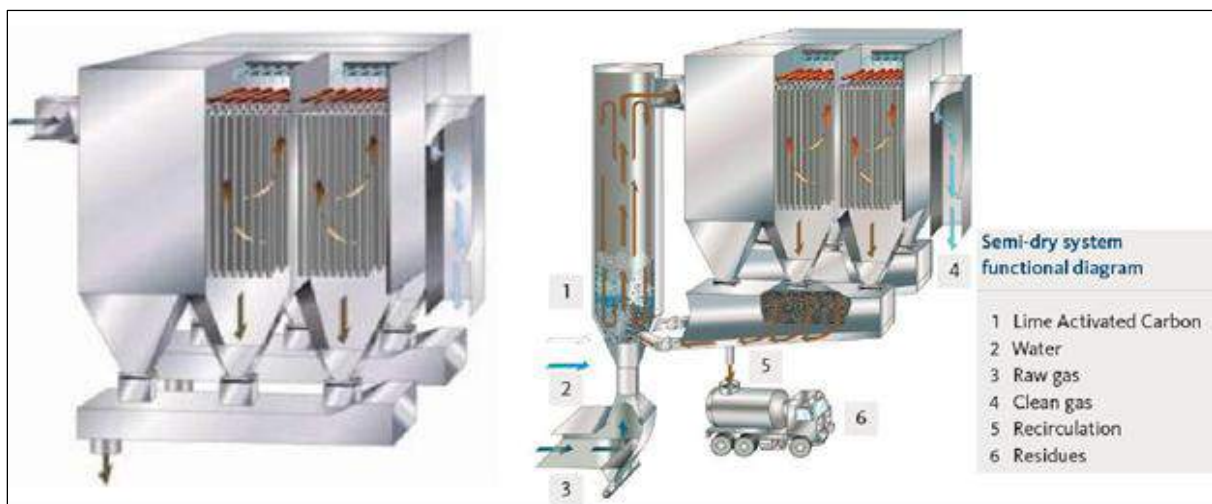
Figure No. 7.13 Semi - Dry Reactor
