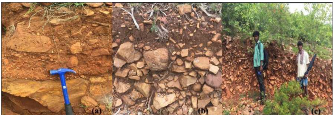
Figure 3.18: Nature of overburden in pediment zone extending between cliff and low lying flat area near to Proposed Power House area
