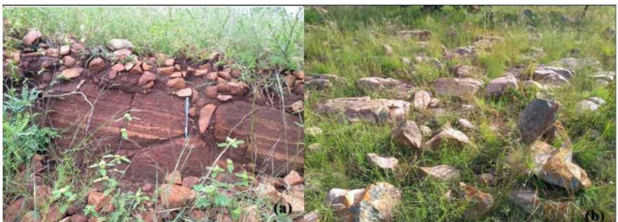
Figure 3.14: Thin scree material over the bed rock (a) & rock blocks/boulders of quartzite occurring at the top
