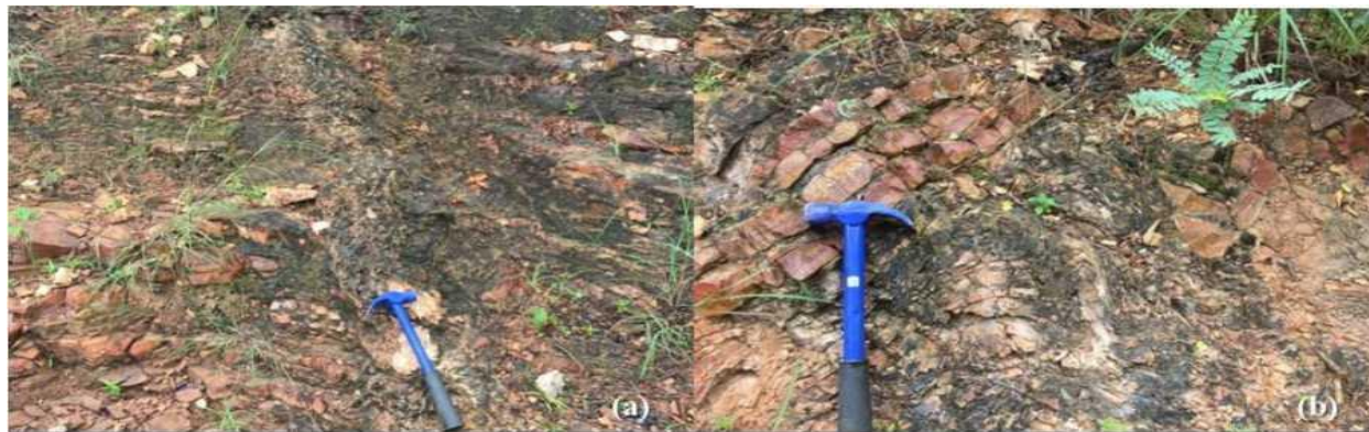
Figure 3.11: Upright, open folds developed in interbedded sequence of sandstone-shale occurring over the moderately weathered granite
