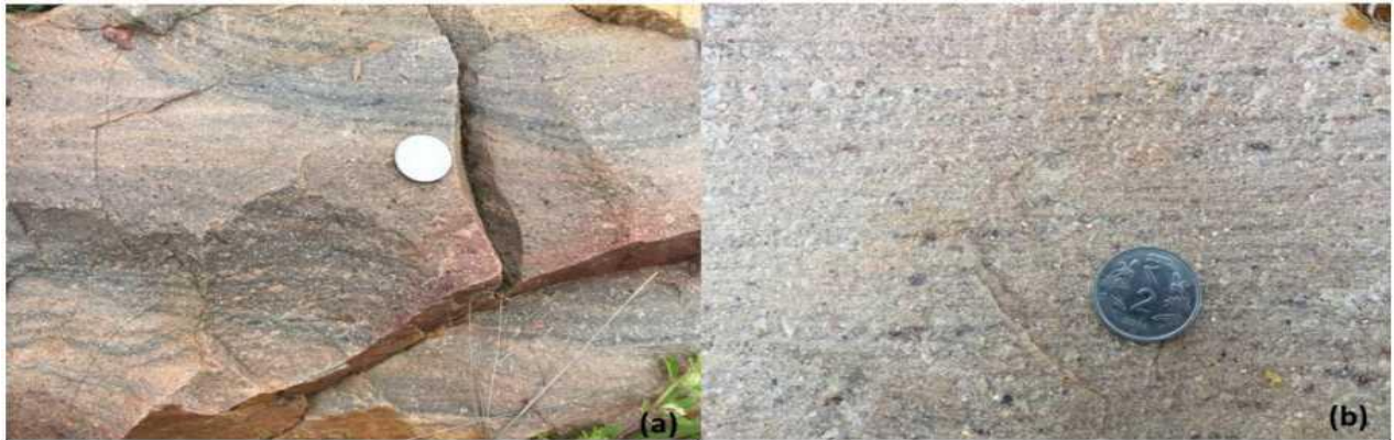
Figure 3.15: Bedding planes in quartzite represented by colour laminations and variation in grain size
