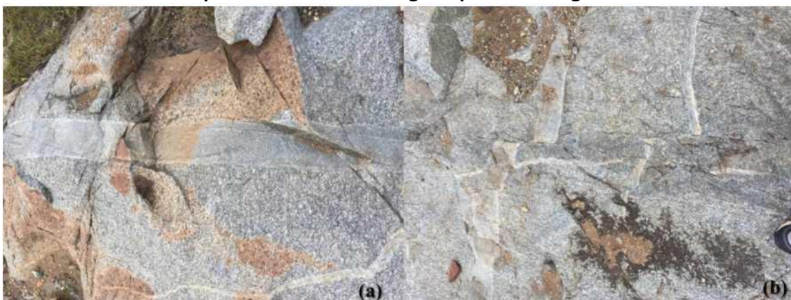
Figure 3.20: Fresh granite rock may intercept in Power house area after crossing of weathered granite profile.
