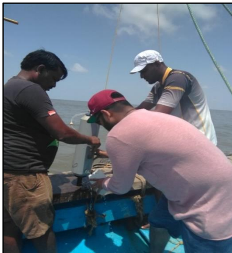
Marine Water Sampling using NISKIN Sampler
