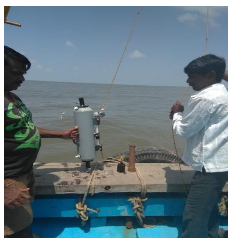
Marine Water Sampling using NISKIN Sampler
