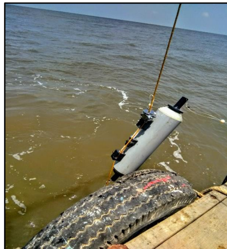
Marine Water Sampling using NISKIN Sampler
