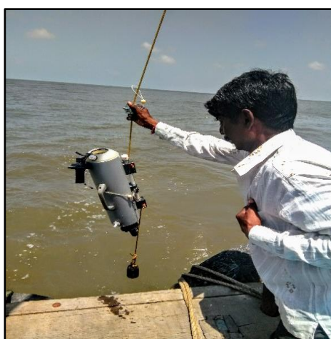
Marine Water Sampling using NISKIN Sampler
