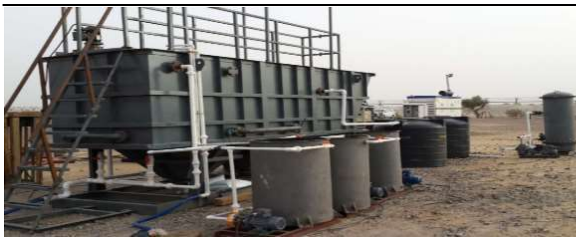
Figure 2.19 A Typical skid mounted Mobile Effluent Treatment Plant
