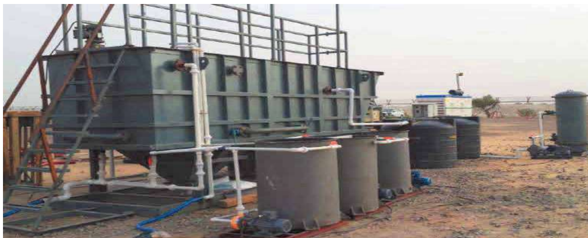
Figure 1.2 A Typical skid mounted Mobile Effluent Treatment Plant
