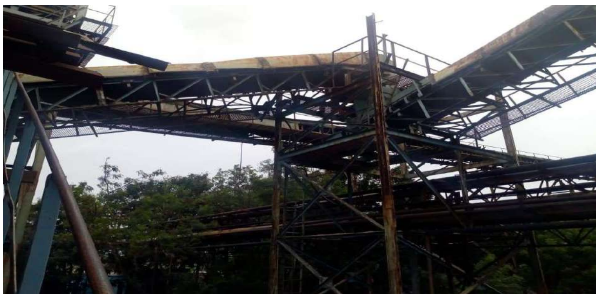
Bagasse Carrier Belt covered by hood to avoid the fugitive dust
