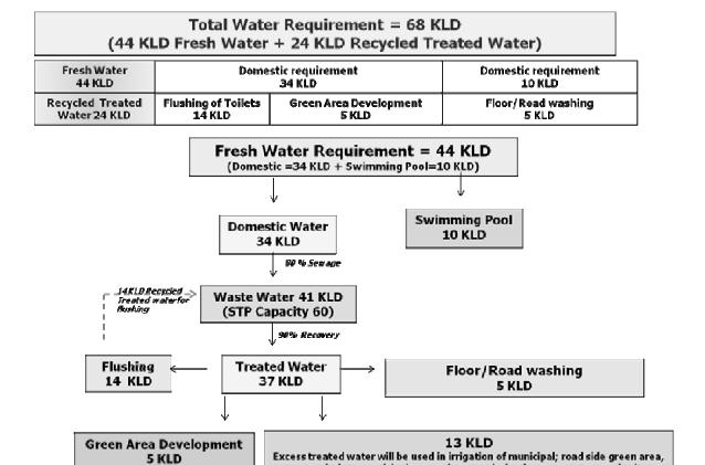
The fresh water requirement of the project will be reduced by adopting above said water conservation measures & using treated water. The waste water generated in the form of sewage will be treated in STP and reutilized in flushing of toilets & green area development / plantation.
