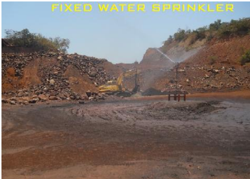
Dust Suppression System at Hopper
