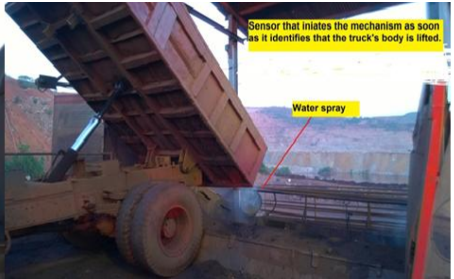
Dust Suppression System at Hopper
