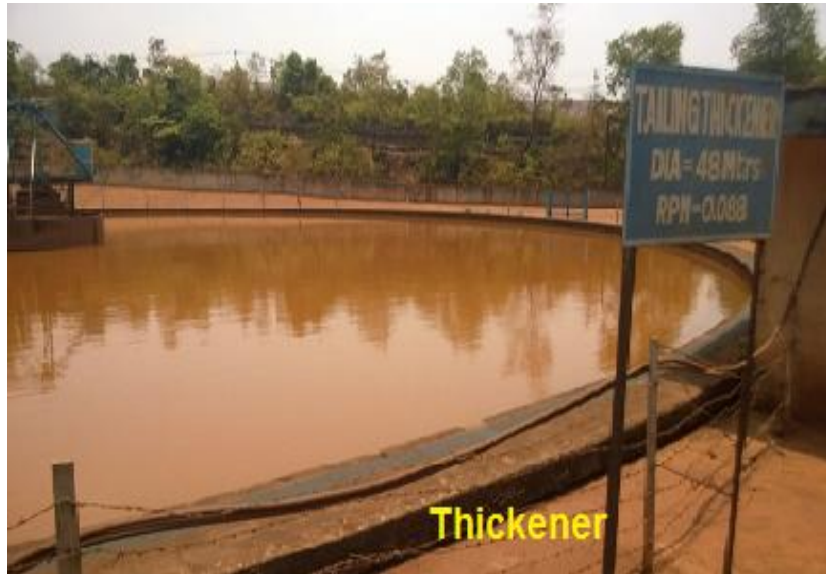
Thickener and Water Recirculation Arrangement
