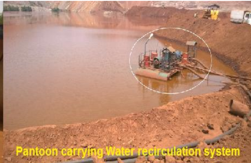
Thickener and Water Recirculation Arrangement
