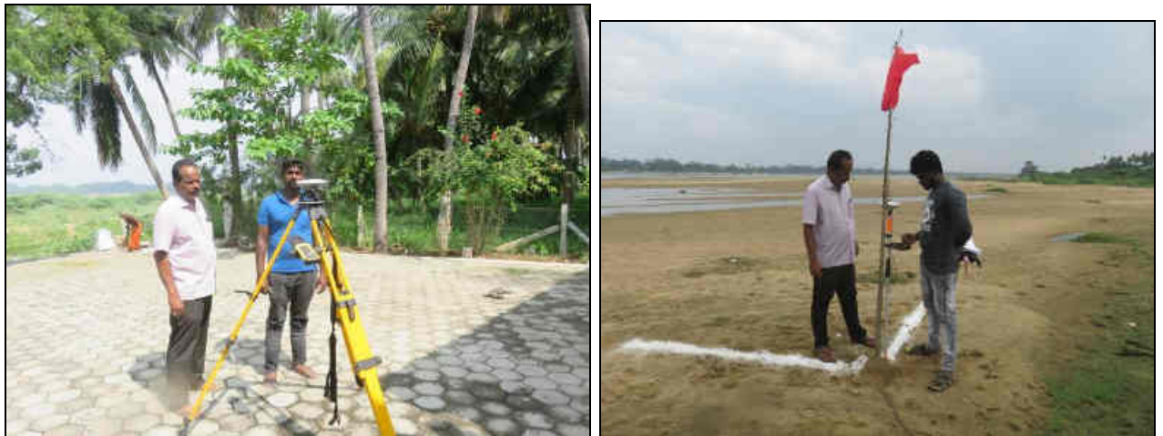
Fig.3. 2 DGPS survey for Ground control Points (GCP) and Drone for Aerial surveying
