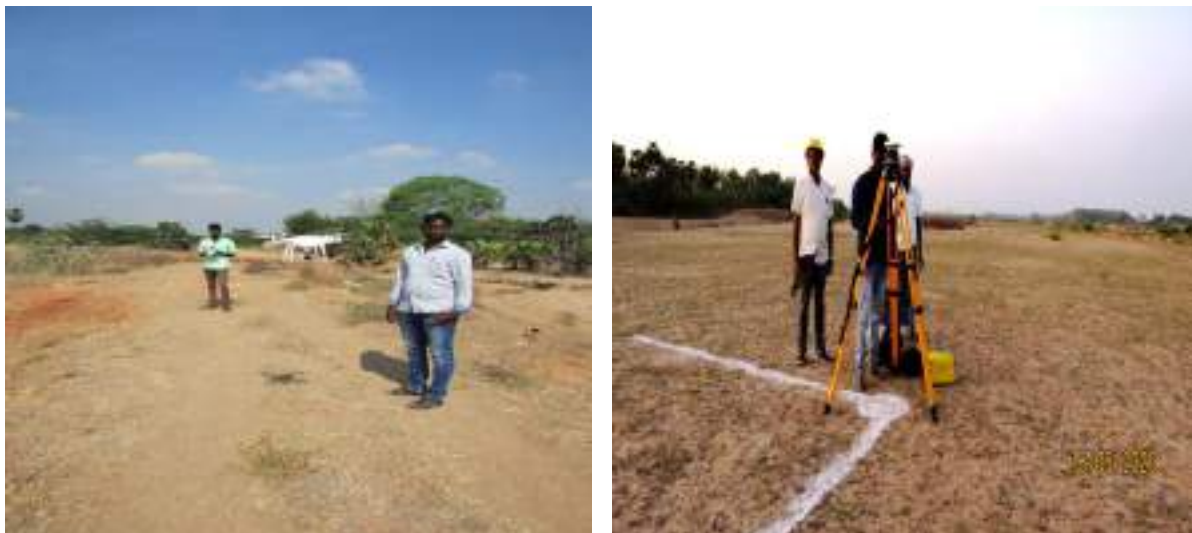
Fig: 2. DGPS survey for Ground control Points (GCP) and Drone for Aerial surveying
