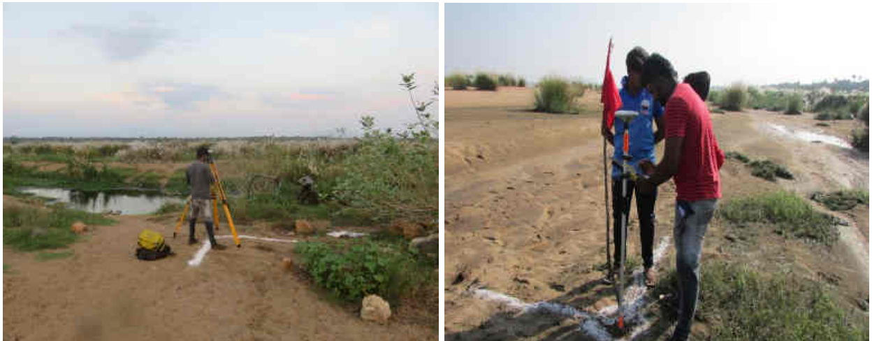
Fig.3. 2 DGPS survey for Ground control Points (GCP) and Drone for Aerial surveying
