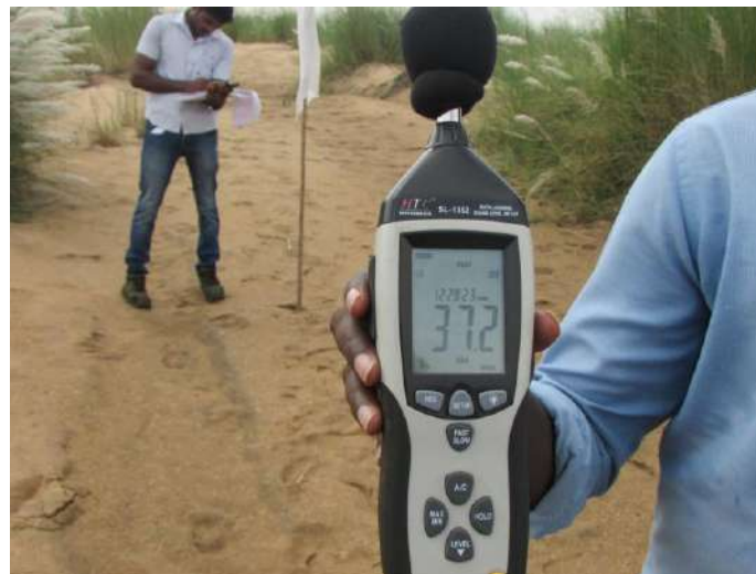
• Fig: No: 4: Measuring Noise Level
