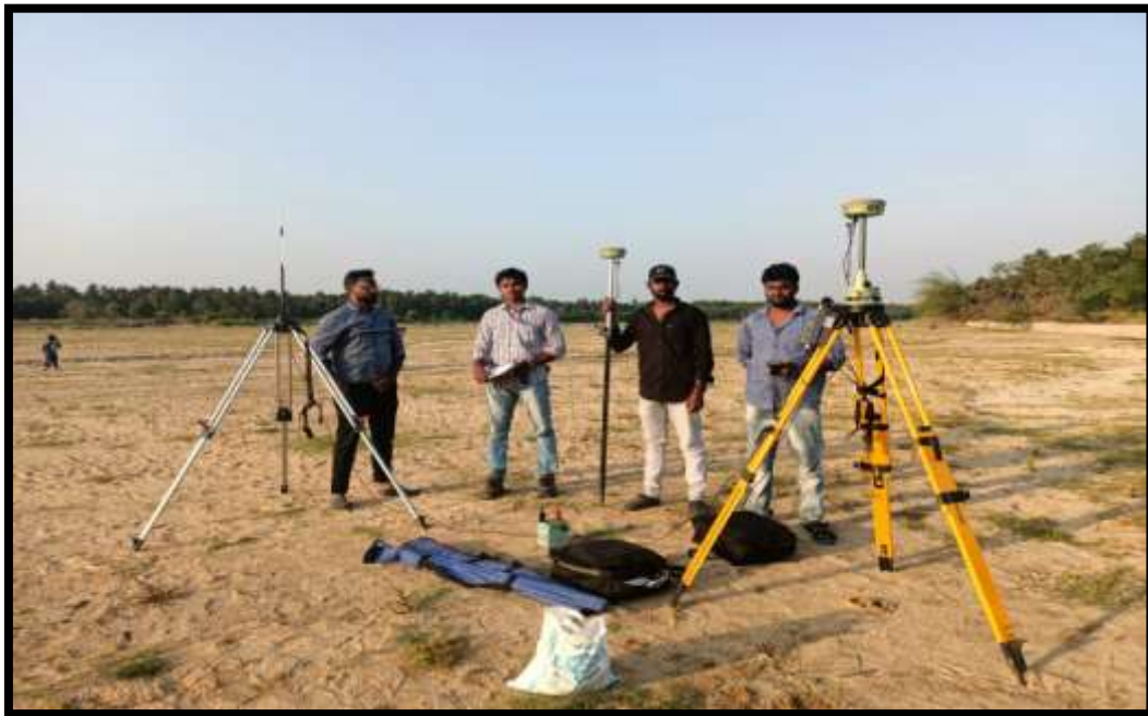
Fig.No.3.2: Photo showing DGPS survey to fix boundary pillars and GCP
