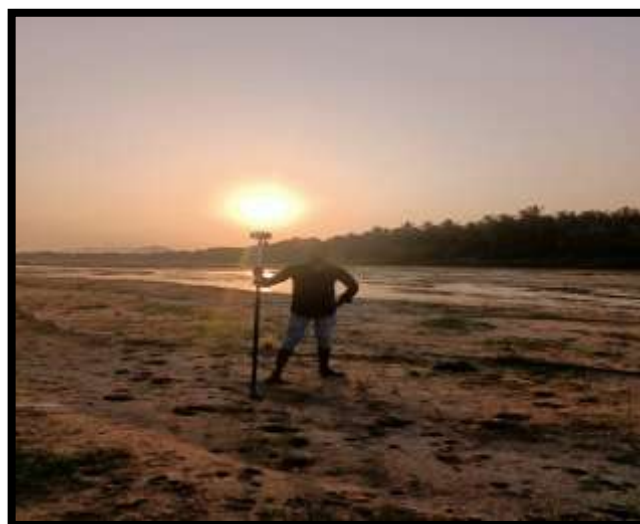
Fig.No.3.2: Photo showing DGPS survey to fix boundary pillars and GCP
